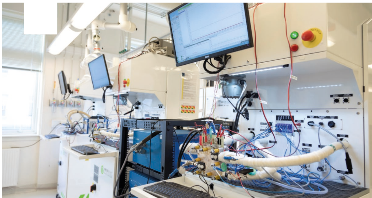
Figure 13 – Testing and evaluation of the performance of PEM fuel cells was a key research activity in MoZEEs (Photo: Norwegian Fuel Cell and Hydrogen Centre, SINTEF, Trondheim).
