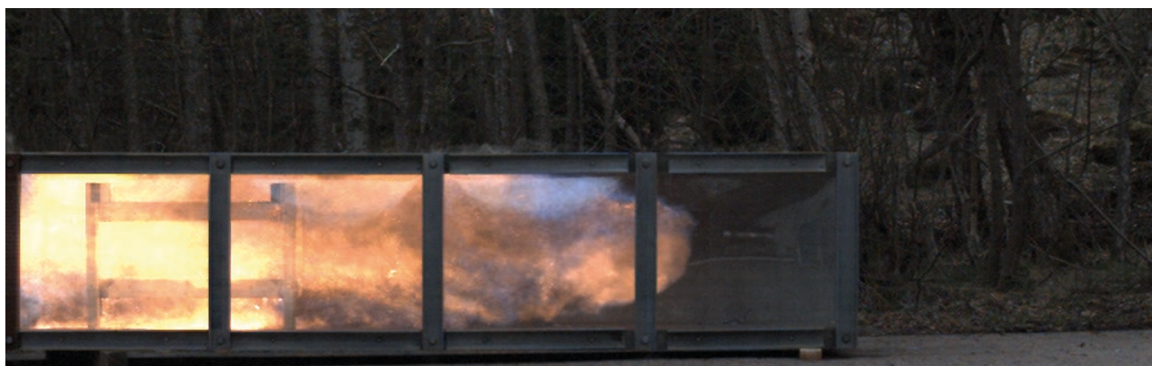
Figure 18 – The 6 meter explosion test rig at FFI was used to study deflagration of hydrogen gas mixtures using high speed cameras, with and without barriers and/or obstructions (Photo: USN).
