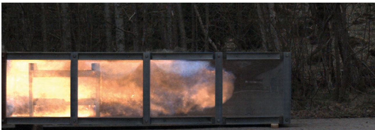
Figure 3.3: Deflagration of an ethane-hydrogen mixture in the 6 meter channel.
