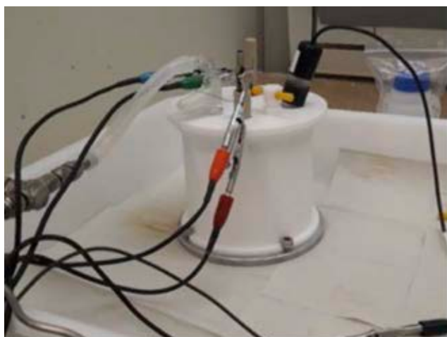
Figure 3. Experimental set-up used for testing activated stainless steel electrodes for alkaline water electrolysis (left) and cell voltage with activated stainless steel and nickel electrodes (right).
