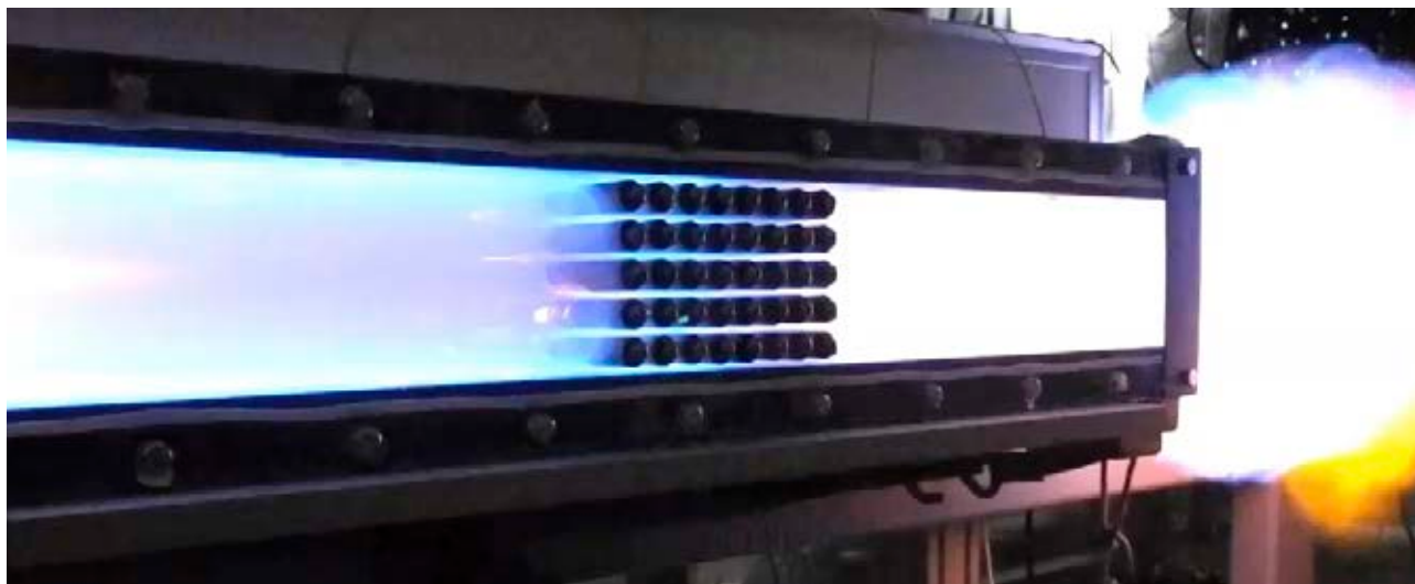
Figure 4: Picture from flame propagation experiment in 1 m explosion channel with obstructions at USN.
