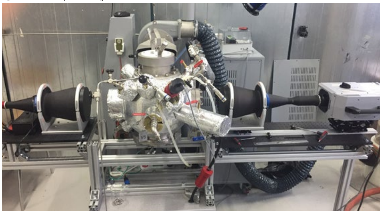
Figure 2: The 20-liter explosion test rig at USN
