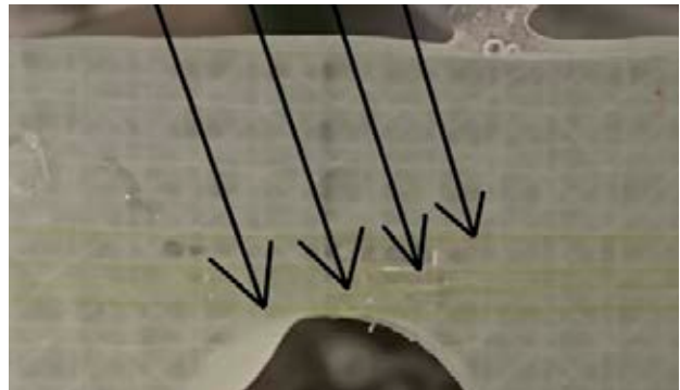
Figure 4: Optical fibers glued onto a flat specimen.
