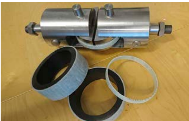
Figure 3: Split disk test rig with a pressure vessel cut out installed. The two cut outs with the black ring inside has not got the liner removed yet. The liner can be seen as the winding mandrel in Figure 1.
