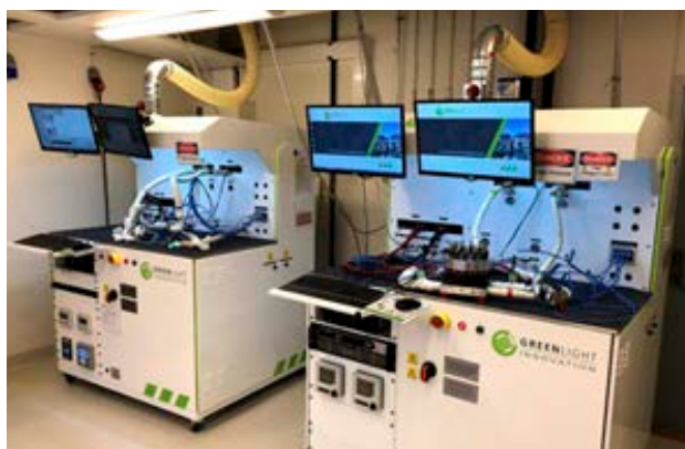
Water electrolyzer cell and stack test stations commissioned at SINTEF, Trondheim
