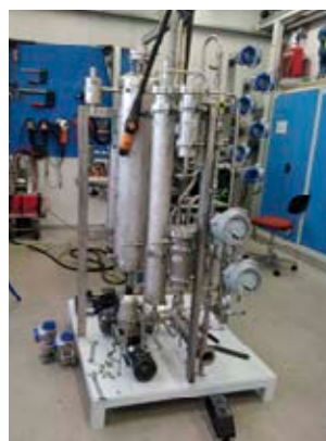
High-pressure PEM water electrolyzer test rig under construction at IFE
