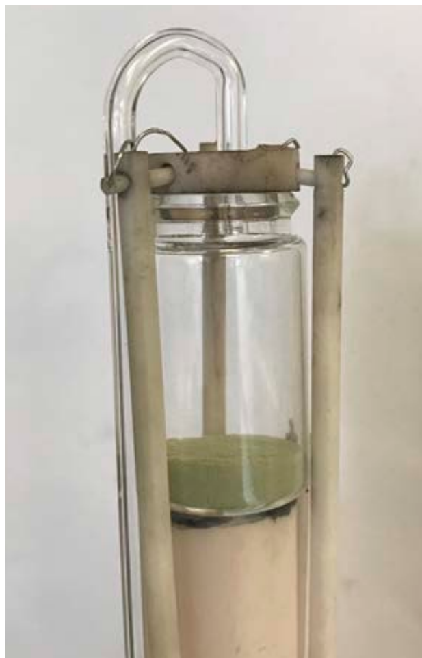
Oxide powders mounted in apparatus for reductive treatment in Task 2.1.
