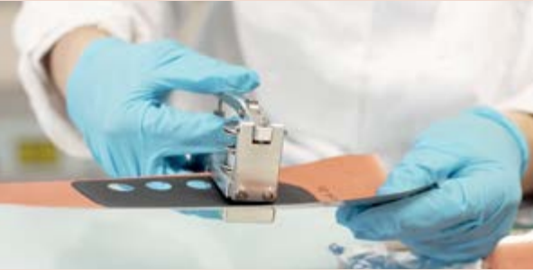
Fig. 1. ▶ Precise puncher is used to cut out disc-shape electrodes formed on Cu foil.
