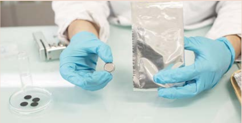
Fig. 2. ▶ A coin cell is a single-cell battery with capacity typically < 300 mAh. A pouch cell (right) can be made of several electrode sheets, and can reach capacities hundred times that of a coin cell due to the larger size, and (if used) additional electrodes sheets.
