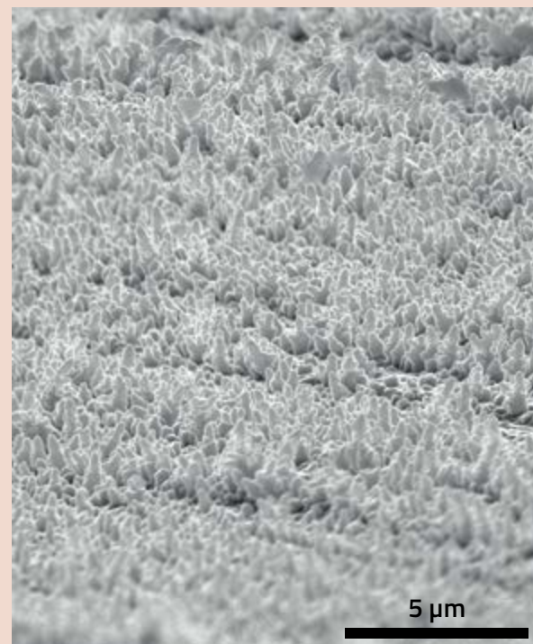
Fig. 2. Copper foil with dendritic pillars.
