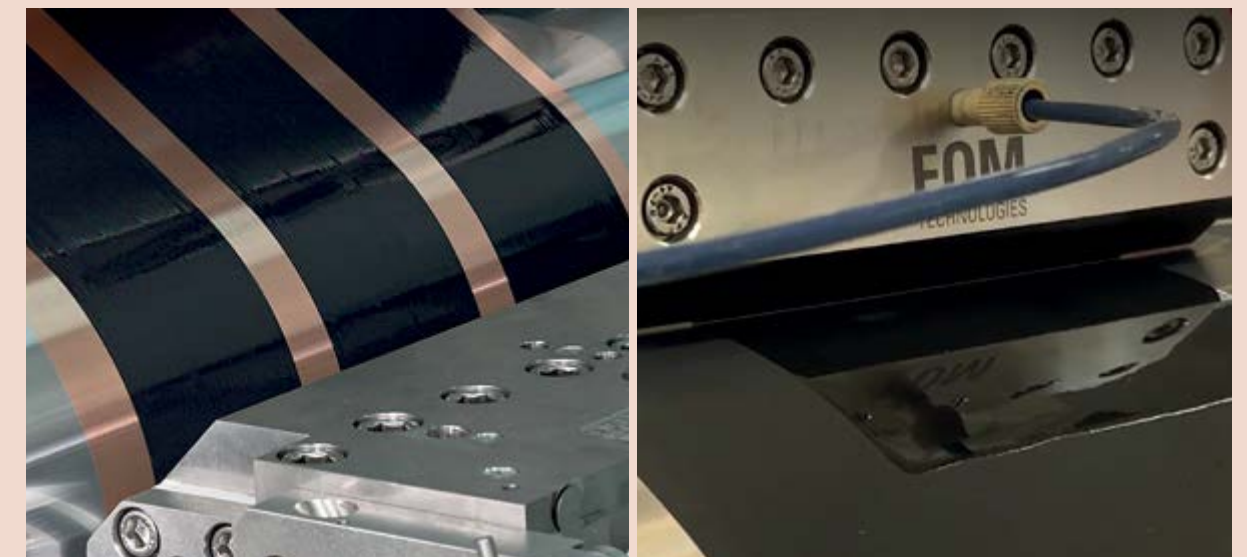
Fig. 2. Graphite-based slurry being coated on carbon film (left). Silicon/graphite composite layers formed on copper metal collector (right).
