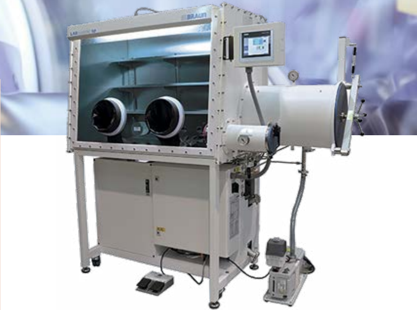
MBRAUN LABmaster pro GLOVEBOX with Vacuum oven
