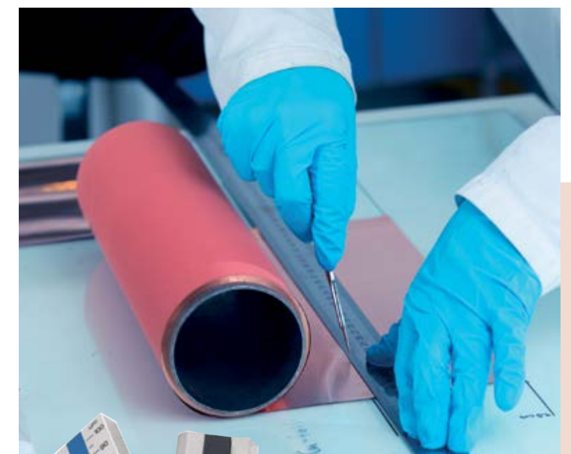
Fig. 1. Current collector (Cu foil) is cut by hand using a scalpel.
