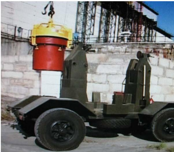
Example: Remote operated equipment for removal of highly contaminated wastes during removal of the “pioneer wall” from the accident liquidation time to prepare NSC erection.
