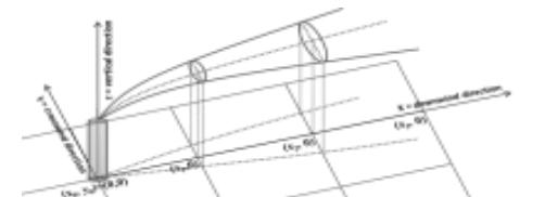
$$C(x, y, z) = \frac{Q(x)}{2\pi \cdot \sigma_y(x) \cdot \sigma_z(x) \cdot u_{10}} \exp \left[ \frac{-y^2}{2\sigma_y(x)^2} \right] F(x, z)$$
