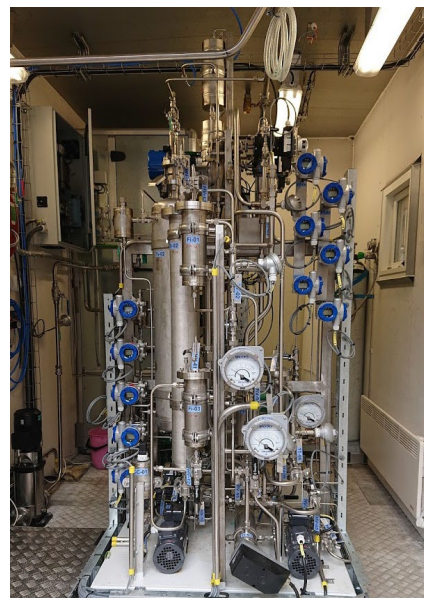
Flexible BoP with adjustable hardware Pressure vessels/tanks, coolers/dryer, filters/mix-beds all designed and built by IFE.
