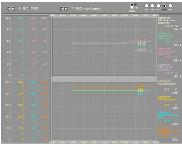
Figure 6: Two historic trend diagrams on top of each other, each diagram displaying four curves. Individual scales for each curve at the left.
